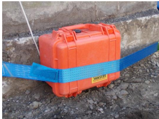
(2) Sensor Attached to Structure
