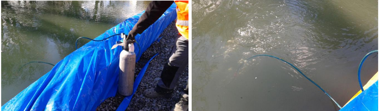
Testing of the CO 2 diffuser
