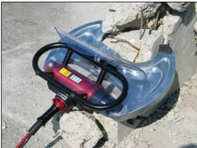
Concrete approach: A remotely operated hydraulic jaw crusher has proved invaluable for tight spaces.
