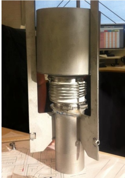
Figure 1: Steinhardt HydroFlush Device without outer casing
